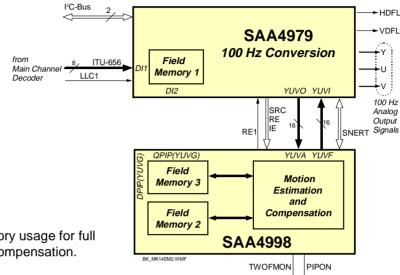
Fig. 83 Data flow and memory usage for full motion estimation/compensation.
