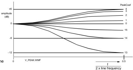
Fig. 81 Frequency response of the vertical peaking function
