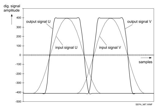
Fig. 50 DCTI with separate processing of both signals (separate = 1)
