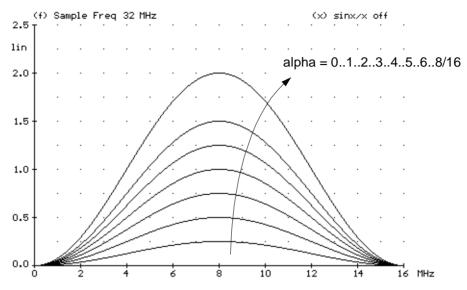
Fig. 53 Frequency response of the peaking band pass filter 2
