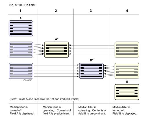
Fig. 4 Median filter used to generate interpolated pictures
