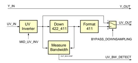
Fig. 35 Block diagram of the output part of the expansion port
