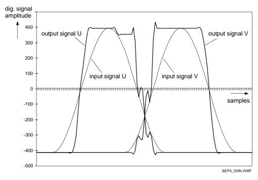
Fig. 49 DCTI with common processing of both signals (CTI\_SEPARATE = 0)
