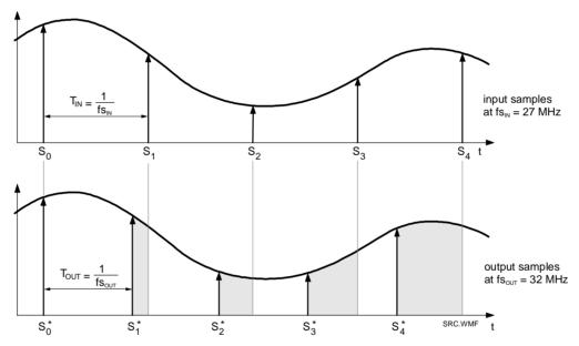
Fig. 34 Sample rate conversion by interpolation
