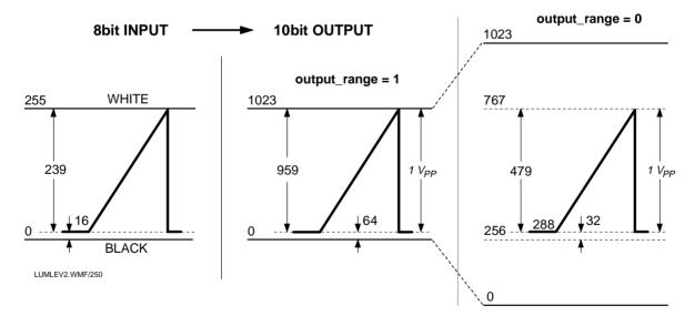
Fig. 58 Input / output signal levels of luminance signal
