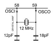
Fig. 65 Application diagram of Crystal for PLL
