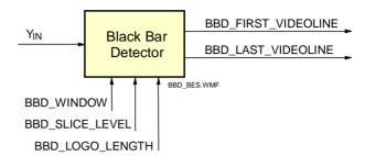
Fig. 26 Block diagram of the black bar detection
