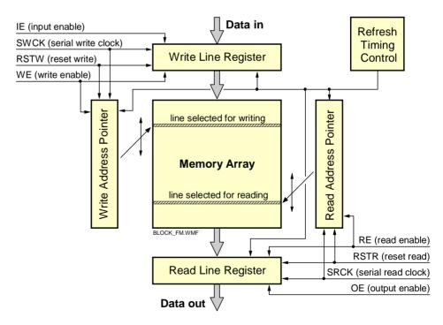
Fig. 1 Block diagram of the scan conversion field memory
