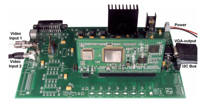
Fig. 92 IPQ board MK14-EM on mother board
