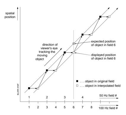
Fig. 67 100 Hz field repetition causes blurring at moving edges
