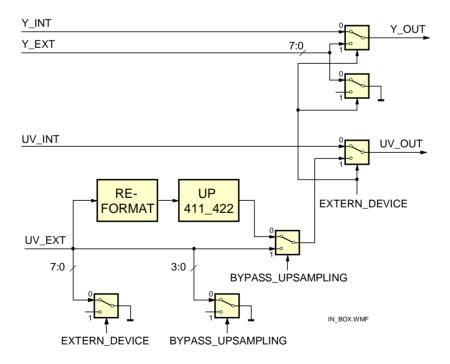
Fig. 36 Block diagram of the input part of the expansion port
