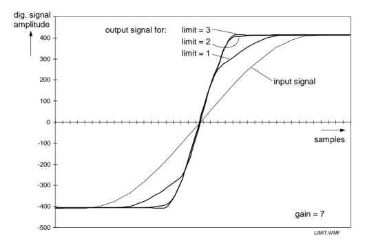
Fig. 42 DCTI with variation of limit for a gain setting of 7
