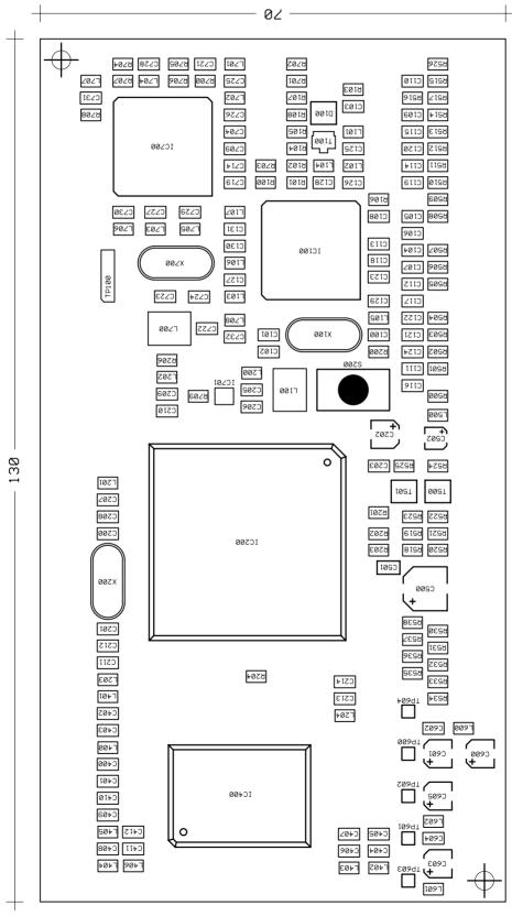
Fig. 105 IPQ module MK14-EM: position of part (top side)
