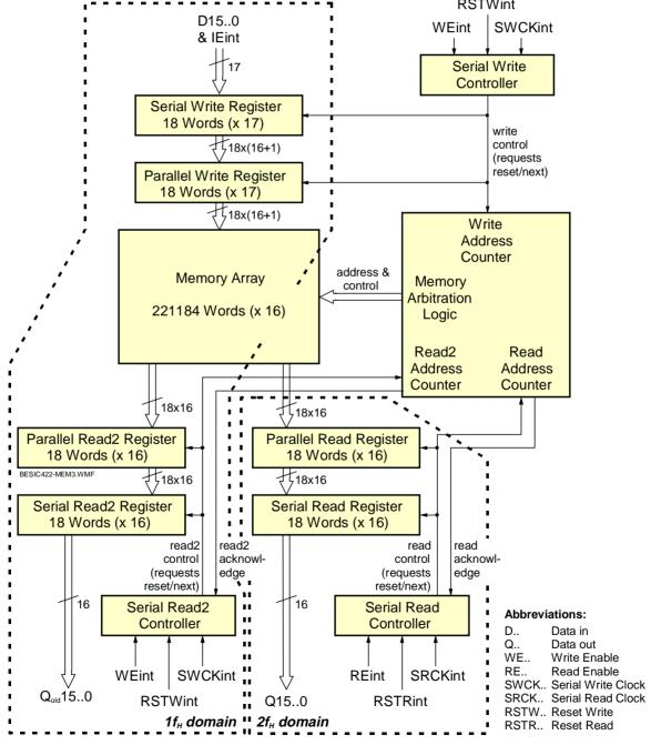
Fig. 33 Block diagram of the scan conversion memory
