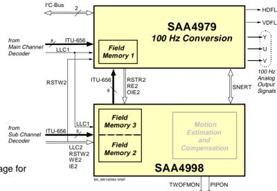
Fig. 85 Data flow and memory usage for highest resolution PIP.
