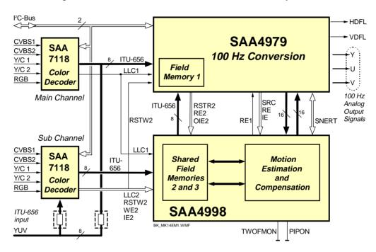
Fig. 89 Block diagram of the MK14-EM module
