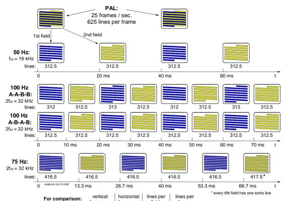
Fig. 12 Format comparison 50 Hz / 100 Hz / 75 Hz
