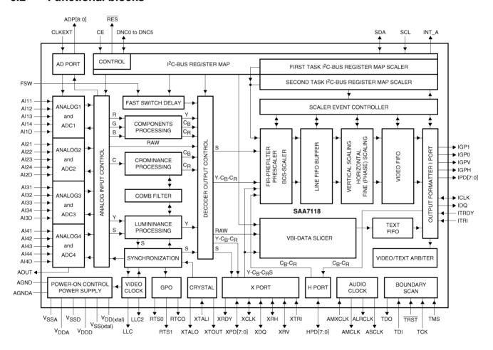
Fig. 88 Block diagram of the SAA7118
