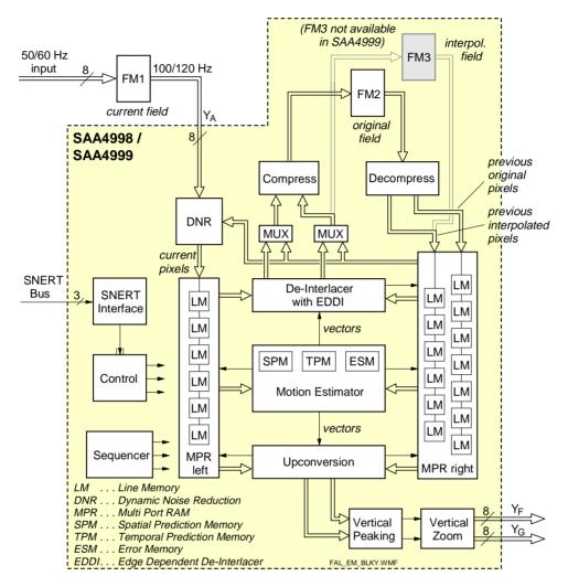
Fig. 69 Block diagram of the SAA4998/..99 luminance processing
