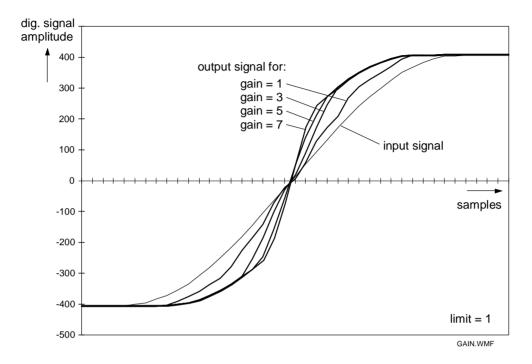
Fig. 41 DCTI with variation of gain for a limit setting of 1
