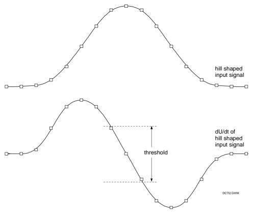
Fig. 43 Principle of hill detection
