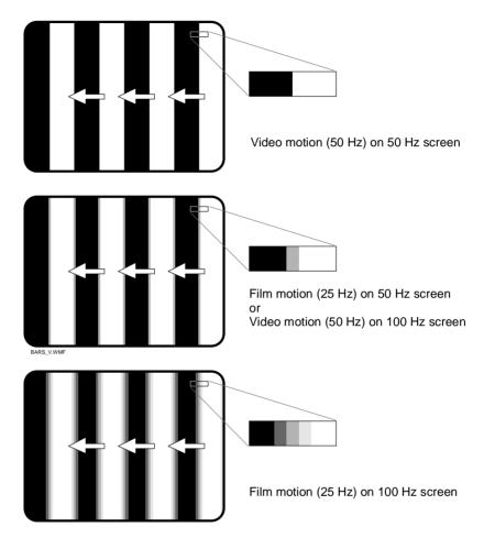
Fig. 5 Moving bars: motion artefacts along the edges
