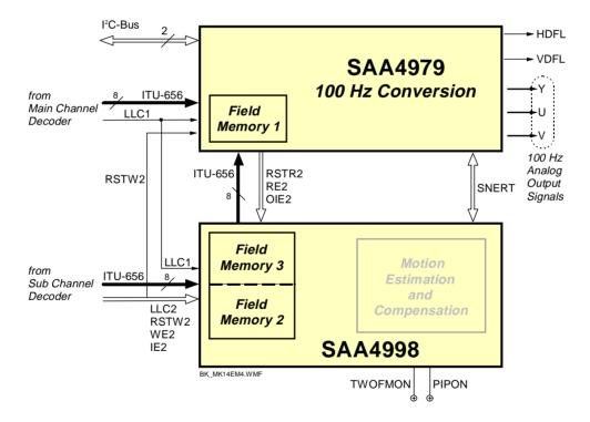
Fig. 94 Data flow in two-channel display mode
