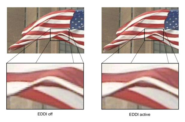
Fig. 79 Removing deinterlacing artefacts with EDDI
