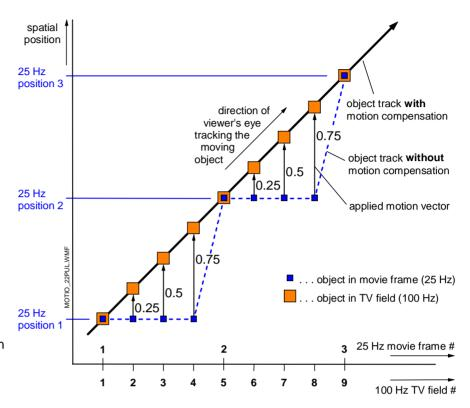
Fig. 9 Motion compensation in 2:2 pull-down movie mode
