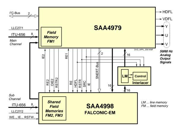
Fig. 95 Block diagram of motion compensation in a DVD player
