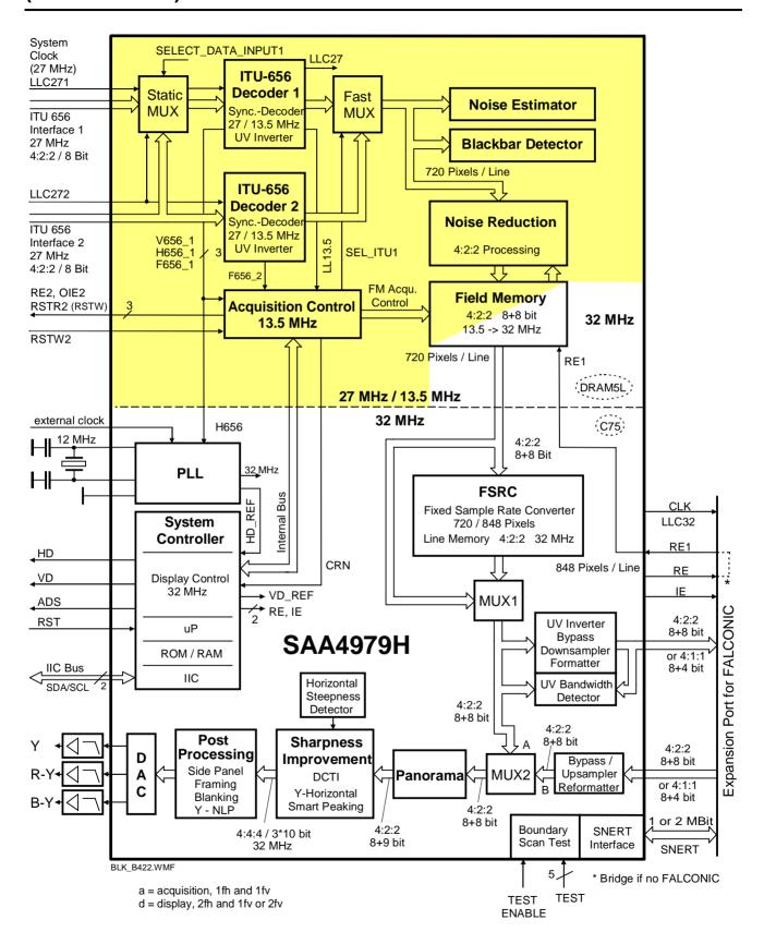
Fig. 17 Block diagram of the SAA4979H
