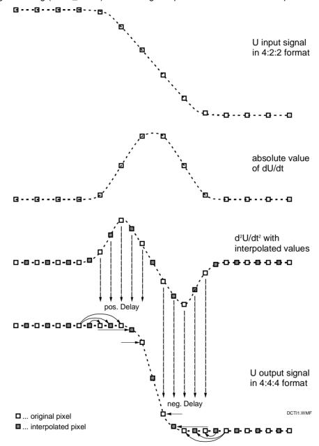
Fig. 39 DCTI basic operating principle
