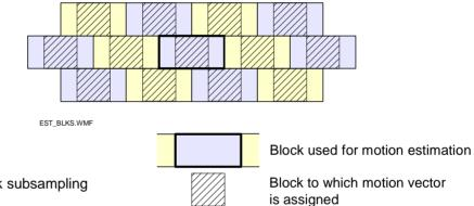
Fig. 70 Motion estimator block subsampling
