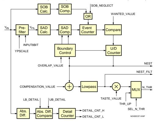
Fig. 30 Block diagram of noise estimator
