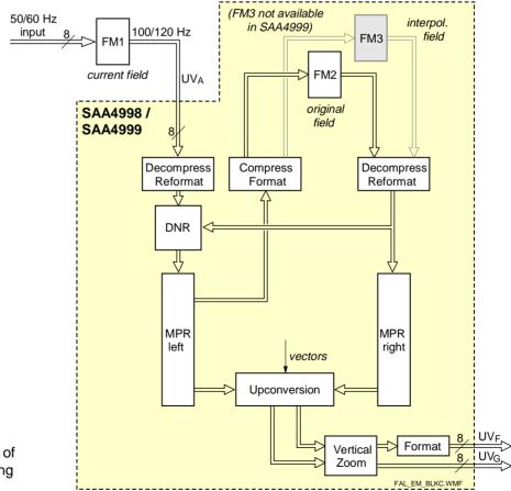
Fig. 82 Block diagram of chrominance processing
