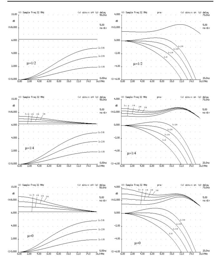
Fig. 59 Group delay and transfer curves of the NLP D/A filter
