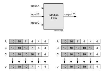
Fig. 3 Function of a median filter
