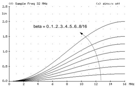
Fig. 54 Frequency response of the peaking high pass filter
