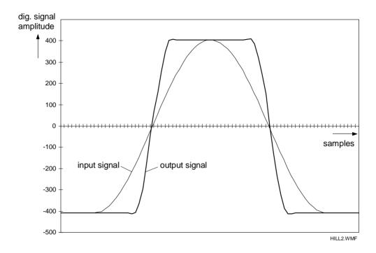
Fig. 45 DCTI with over-the-hill-protection
