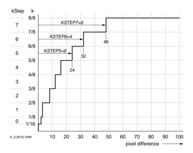
Fig. 28 Sample noise reduction k-curve
