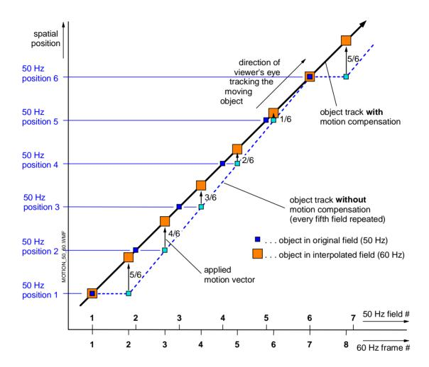
Fig. 15 Motion compensation in 50i/60p conversion mode
