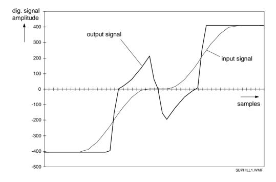
Fig. 46 DCTI with superhill-protection off
