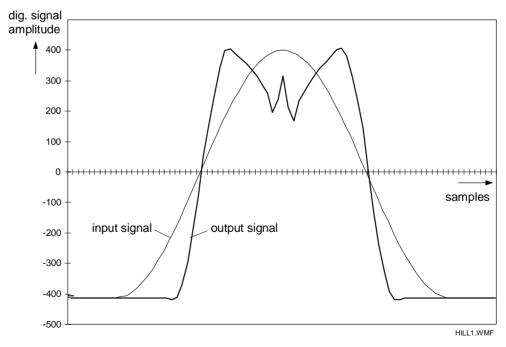
Fig. 44 DCTI without 'over-the-hill protection'
