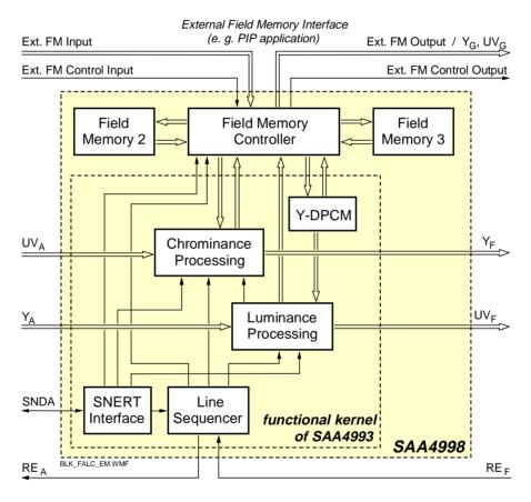
Fig. 66 Block diagram of the SAA4998
