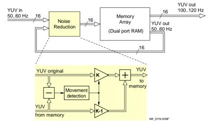
Fig. 27 Basic block diagram of the DNR circuit
