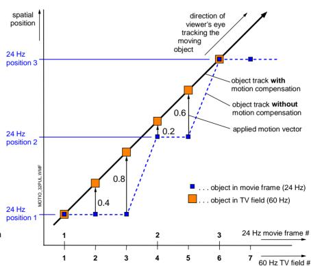
Fig. 10 Motion compensation in 3:2 pull-down movie mode
