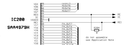
Fig. 91 Running the MK14-EM board without subchannel and motion compensation.
