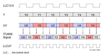
Fig. 18 ITU-656 multiplex signal
