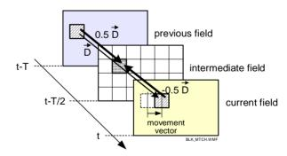
Fig. 68 Block matching principle
