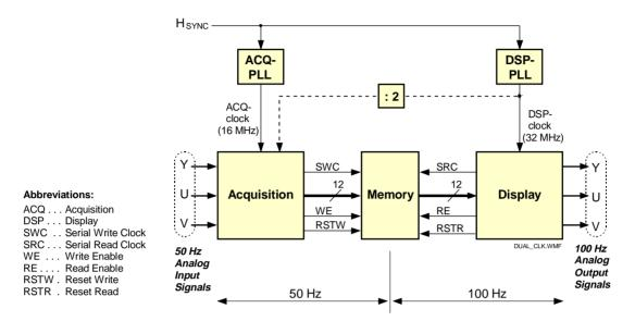
Fig. 16 Single clock and dual clock system in scan conversion
