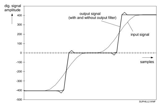
Fig. 47 DCTI with superhill-protection on
