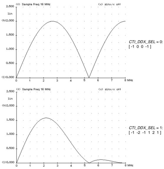
Fig. 40 Transfer curves of the first differentiating filter
