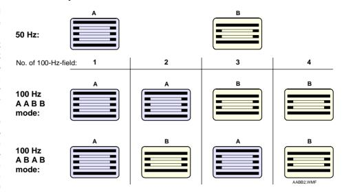
Fig. 2 Scan conversion modes A-A-B-B and A-B-A-B
