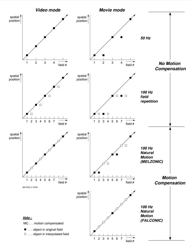
Fig. 6 Scan conversion with and without motion compensation
